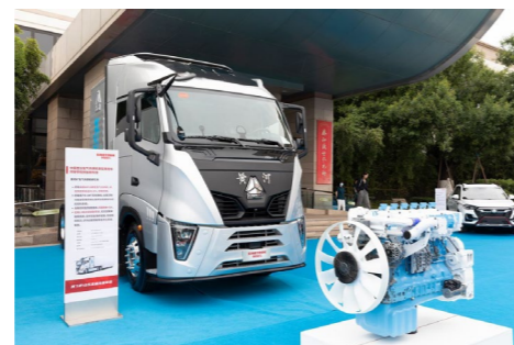
The Yellow River heavy truck with hydrogen internal combustion engine of Sinotruk
